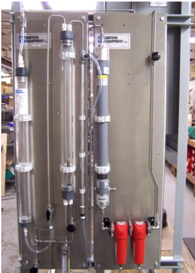
WATERS MODEL W7951-01 SPARGER WITH MODEL W7950-10 NITROGEN GENERATOR
